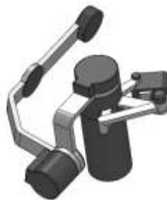
Fig.3 Wrist joint mechanism and holding jaw mechanism
