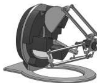
Fig.2 The Delta mechanism of Omega.7
